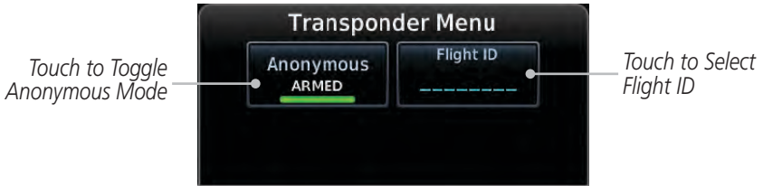
Figure 2-14 ADS-B/Transponder Control Panel
