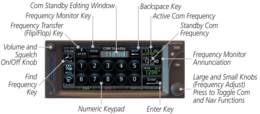
Figure 3-1 Nav/Com Controls
