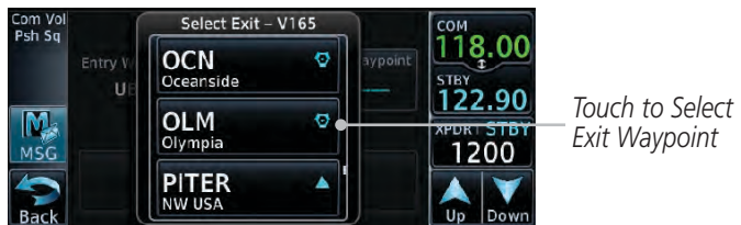
Figure 4-24 Select an Exit Waypoint for the Airway
