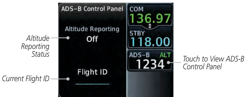
Figure 2-13 ADS-B Control Panel
