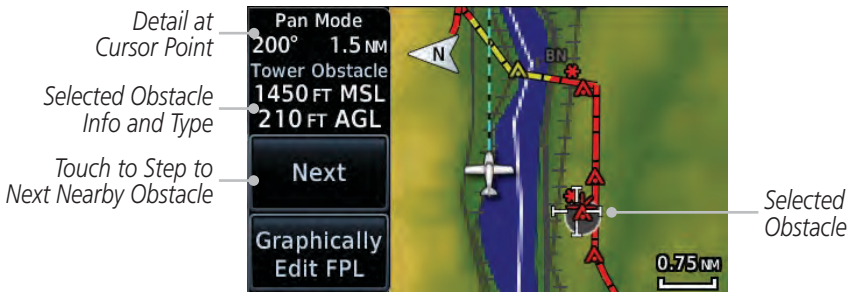
Figure 8-25 Point Obstacle Detail
