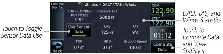
Figure 14-37 Utility DALT/TAS/Winds Page Using Sensor Data and Pressure Altitude
