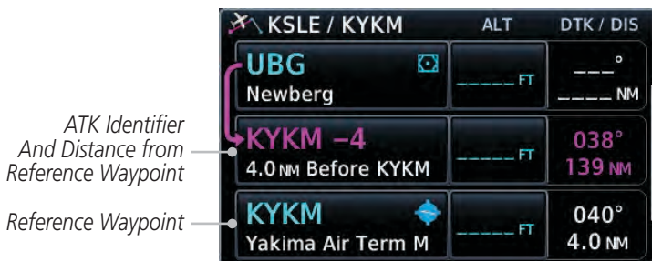
Figure 4-15 ATK Inserted Before Reference Waypoint
