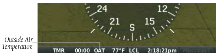
Outside Air Temperature on PFD Status Bar (GDU 46X)
