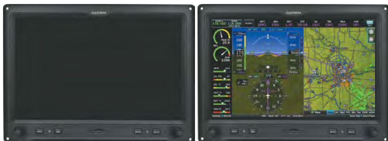
G3X Touch Full-Screen Reversionary Mode (Failed PFD)
