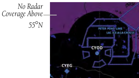
NEXRAD Radar Coverage Limitations
