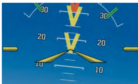
ESP Engaged (Nose-High)
