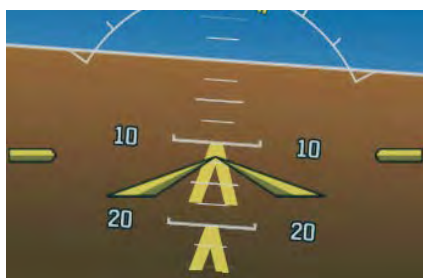
ESP Engaged (Nose-Low)
