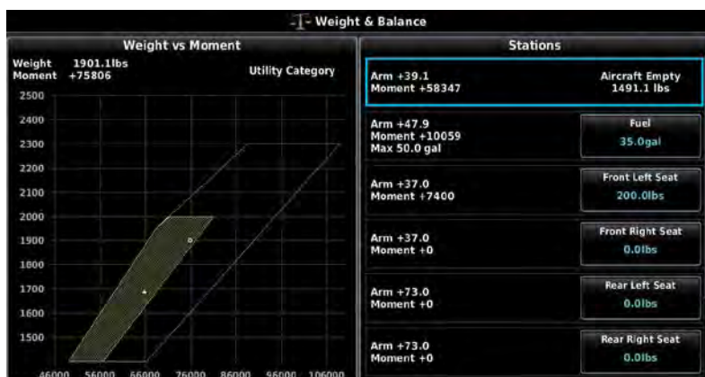
Weight and Balance Page - Weight vs Moment
