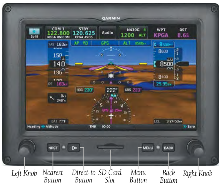
Left Knob Nearest Button Direct-to Button SD Card Slot Menu Button Back Button Right Knob Bezel Overview (GDU 46X)
