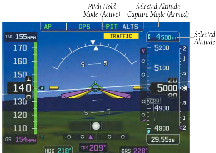
Pitch Hold & Selected Altitude Capture Modes
