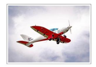
SHARK is powered by a ROTAX 912 ULS 100 hp engine running WOODCOMP 2-blade adjustable propeller. With low operating costs, long range (1600 km), exceptional speed (optimum cruising speed of 140 knots) and long service life, access to any public airport at optimum while keeping operational cost minimum.
